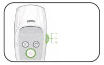
The side push button has three different sound wave modes, which are initiated by 22-25KHZ.
