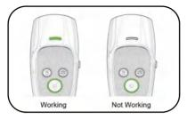
4. First, Try a test to make sure the green indicator light is ON when you press any button, which means the device is working perfectly. If the indicator light does not light up, please contact us at support@nzonpet.com. The professional customer service team will have a dedicated customer service staff to solve it.
