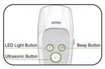
Green indicator light: The green indicator light is for responding to every device's activity if it counts. The indicator light will not blink if any action does not count.
